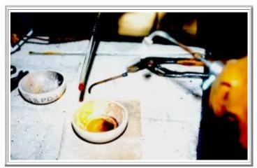
What one must bear in mind are not only the melting point of zinc, 419°C, but also the boiling point of 907°C, the boiling point being below the melting point of any of the other constituents (Figure 10). At the point of volatilisation of zinc, any oxygen present will combine with the zinc and produce white zinc oxide fumes. I found zinc oxide to be a major cause of porosity problems. If not kept to a minimum, zinc oxide remains in the metal and leaves random porosity in any part of the casting.
