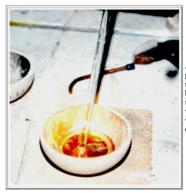
As the alloy is approaching it's pouring temperature, the metal needs stirring to be sure of a homogeneous mix. If using a stirring rod, this is best done with a soda glass, or Pyrex rod, which will also collect any excess flux.
